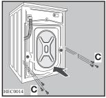
Open the porthole, take out the inlet hose from the drum and remove the polystyrene block fitted with the adhesive tape on the door seal.
